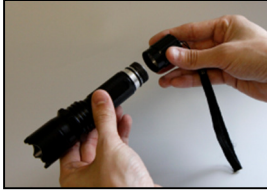
a) Unscrew and remove the rear of the UV torch.
