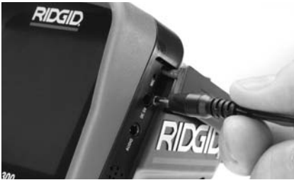
Figure 7 – Powering the Unit with AC Adapter
