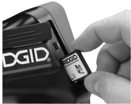
Figure 10 – Inserting the SD Card
