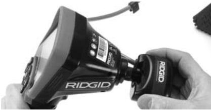
Figure 19 – Camera Connector Plug Installed
