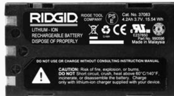
Figure 23 – Label on Battery
