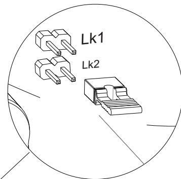
To access speed mode make sure link 1 is fitted.
